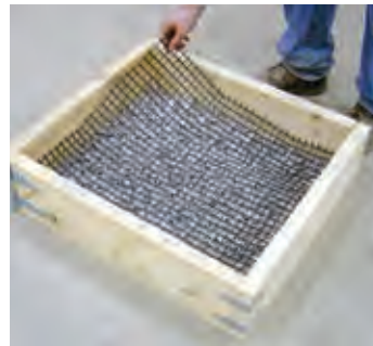
Geo-grid is added between layers of gravel.
