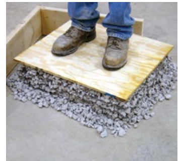
When the walls are removed the layers of Geo-grid maintain the shape of the gravel block.
