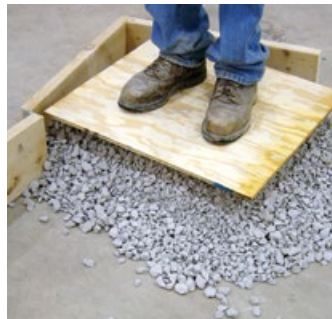
Without reinforcement the gravel collapses when the walls are removed.
