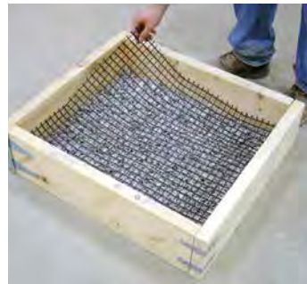
Geo-grid is added between layers of gravel.
