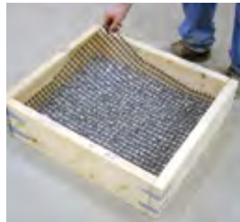
Geo-grid is added between layers of gravel.
